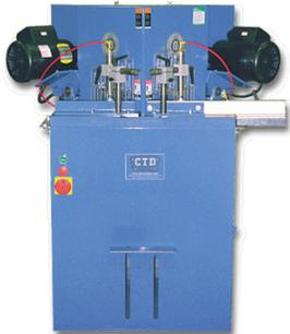
The D45FX is popular world wide for its unique features, low cost and precision. Engineered for high production, this foot operated saw makes two 45 degree mitres at one time, saving time and materials. Available in 10", 12" or 14" blade capacity. Super Duty 1 1/2 H.P. totally enclosed fan cooled motors are available as single or triple phase. Many options are available to maximize your productivity.
