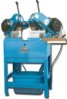
A revolutionary idea-right and left saw heads, individually operated on a single base. Gives you a fast, accurate double mitre cut-off at an affordable price. Features: Heavy duty 1HP fan cooled motors, 12" blade capacity, Solid steel floor stand with removable dust/scrap drawer. Rabbit measuring scale included.
