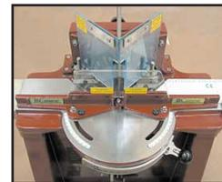
This Mitre Guillotine has been developed to give the gallery picture framer and volume framer both speed and quality cutting. The foot pedal operation brings the blades down to chop through the moulding producing 2 opposite mitres. A re-positionable cutting head allows you to advance the blades and chop through the moulding as many times as is needed to provide the best quality cut. Comes with one set of blades. Secondary sets are recommended for continuous operation during blade sharpening.
